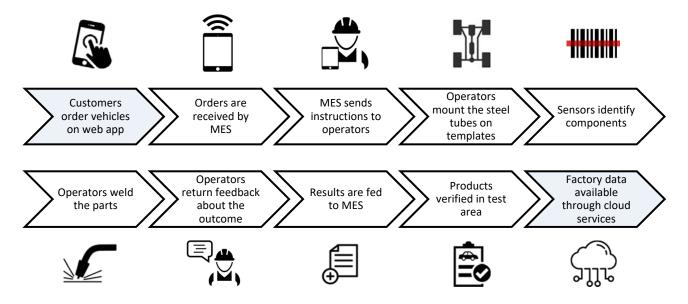
With that kind of manufacture all subcomponents and all assembly processes have to be marked and recorded to allow tracking. A vehicle has to be associated to a specific moment of manufacturing of all its components and subcomponents.
